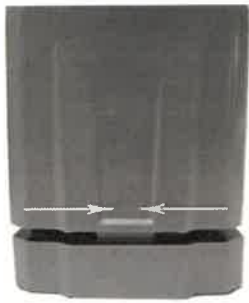
Figure 40: Push at center of endpoint base to release the cover
