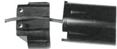
Figure 18: Threading cable harness
